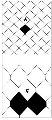
Figure 1. Schematic view of stent-cell designs: (\*) – closed-cell design vs. (#) – open-cell design
