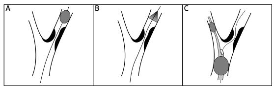
**Figure 3.** Schematic review of emboli protection devices. Guidewire threaded through stenosis of internal carotid artery in all panels. Panel A – distal balloon occlusion device. Panel B – distal filter protection device. Panel C – proximal protection device with distal occlusion balloon (smaller) inflated in external carotid artery and proximal occlusion balloon (larger) inflated in common carotid artery
